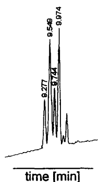
Fig. 4. Electropherograms of a mixture of AQC-Ile and AQC-allo-Ile. Peaks not identified by migration times are impurities. Selector concentration: 0.5% (w/v) of \beta -CD polymer; all other experimental conditions as in Fig. 2. Ordinate: absorbance at 245 nm.
